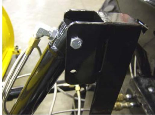
16. Go over all hydraulic connections to ensure there will be no leaks. Fill the pump reservoir full with fluid. Start your vehicle and slowly move the pump in all directions while keeping the pump full of fluid. Do not turn plow with reservoir cap off. Once the system has been worked and the air is out make sure fluid level is still up. Your plow will not work until the fluid bleeds through. Reservoir may leak until fluid seeks its level.
