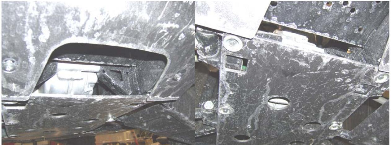
4. Once removed align receiver under vehicle and center over holes. Mark the plastic bumper underneath where trimming of the plastic may need to be done.
