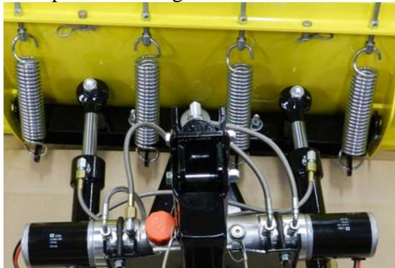
17. Make sure all parts are torqued to spec and your fittings are tight and not leaking. All wiring should be soldered and shrink tubed or black taped.
