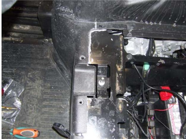
3. Next install the receiver part of the assembly. From under the front of the vehicle, remove the 4 6mm bolts from the plastic skid plate. This should be done with an air ratchet or a power tool of some sort due to some of the nutserts in the frame turning.
